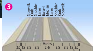
4 Lane Divided – Curb & Gutter on Both Sides
