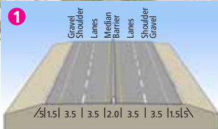
4 Lane Divided – Median Barrier
