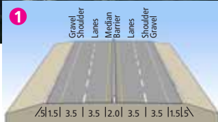
4 Lane Divided – Median Barrier
