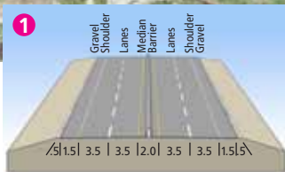
4 Lane Divided – Median Barrier
