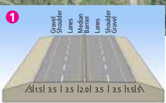
4 Lane Divided – Median Barrier
